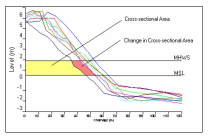
Figure 3.7 Profile Analysis by Level
