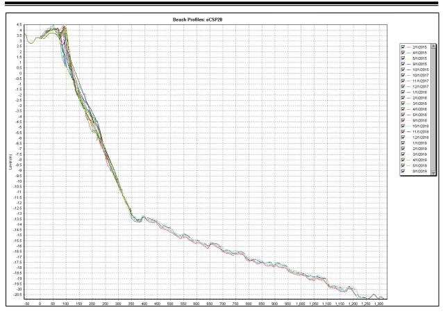
Figure 3.5 Sample beach profile graph of CSP 28 (Pullavila) using SANDS software
