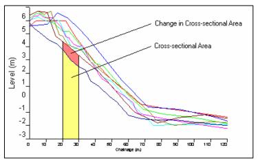
Figure 3.8 Profile Analysis by Chainage
