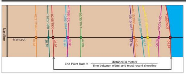
Figure 3.2 Calculation of Short Term Shoreline change analysis (Sample image source: Thieler et al., 2017)
