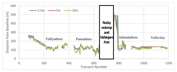
Figure 4.39 Comparison of Shoreline data from satellite images of different spatial resolution and beach profile data with field shoreline
